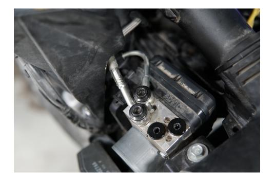
Note: The Rear ABS ports are plugged using the supplied blanking screws.
