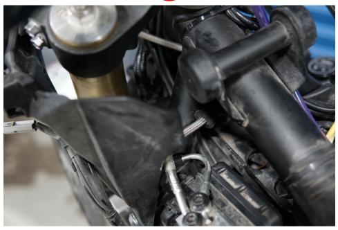
Note: The line is routed through the frame and not between the frame and the fork leg in order to eliminate a pinch risk.
