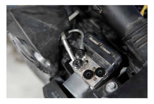
NOTE: The hard line exiting the ABS pump <u>remains in place</u>.
